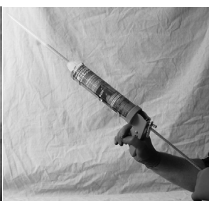
#5 Point gun upright, depress trigger to slowly fill mix tube.
