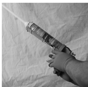
#4 Hold gun upright and place cartridge into it.
